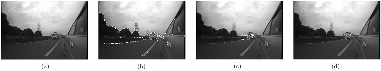
Fig. 6. Detection of approaching side vehicle: (a) Input image, (b) Image detected feature points without limit of processing region, (c) Image detected feature points with limit of processing region, (d) Detected front vehicle region.
