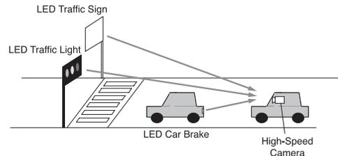
Fig. 1. Road-to-vehicle communication using LED traffic light and high-speed camera.
