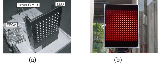
Fig. 6. LED transmitter (a) LED:64 (using FPGA) (b) LED:256
