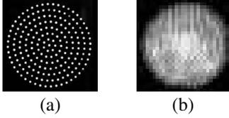
Fig. 4. Image of LED traffic light; (a) Short distance (15m), (b) Long distance (60m).
