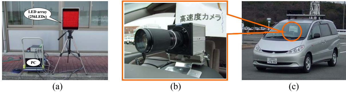
Figure 7. Field trial instruments: (a) LED array transmitter, (b) High-speed camera, (c) Car.
