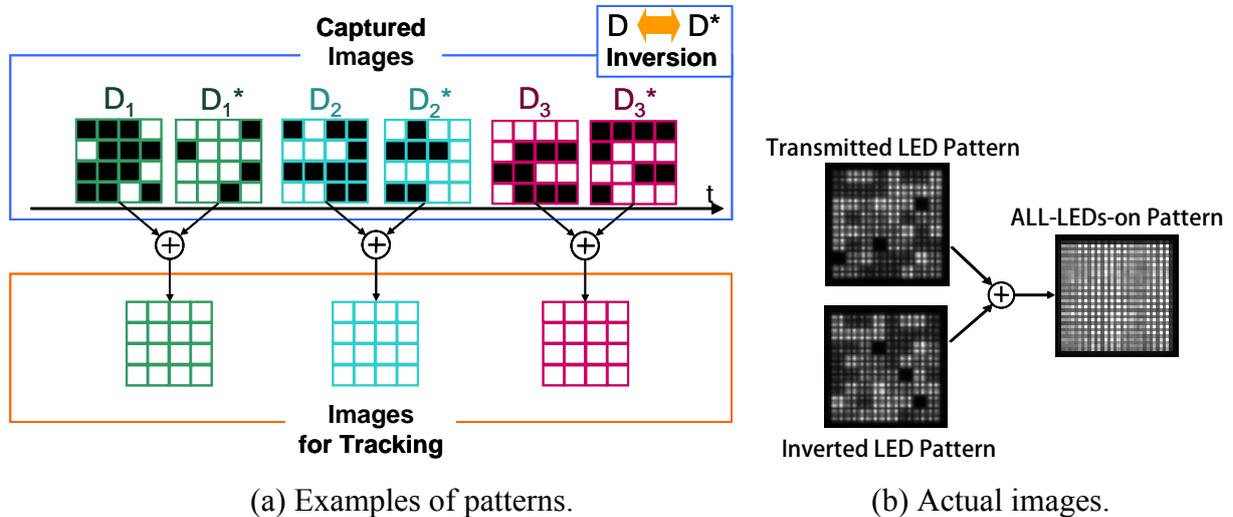
Figure 6. Tracking method using inverted LED patterns.
