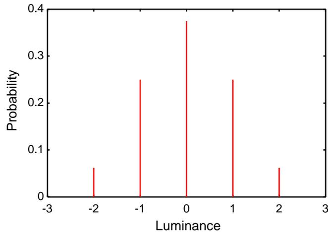
Figure 10. Transmitted luminance ( $x'_{u,v}$ ) distribution of the hierarchical coding.
