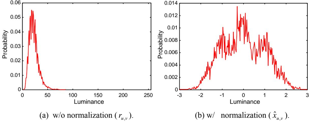
Figure 12. Received luminance distribution at rotation angle  $30^\circ$  (30m).
