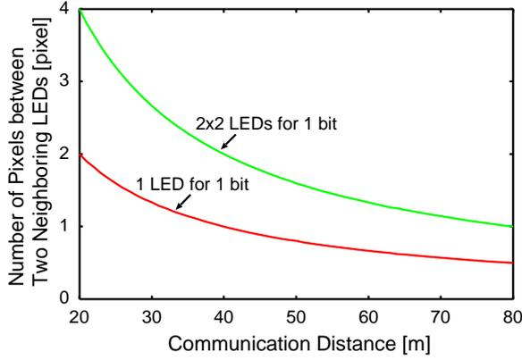
Figure 7. Relation of the communication distance and the number of pixels between two neighboring LEDs
