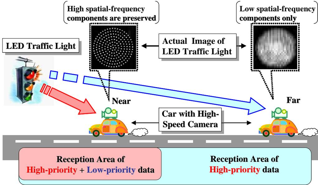
Figure 1. Proposed road-to-vehicle visible light communication (R2V-VLC).
