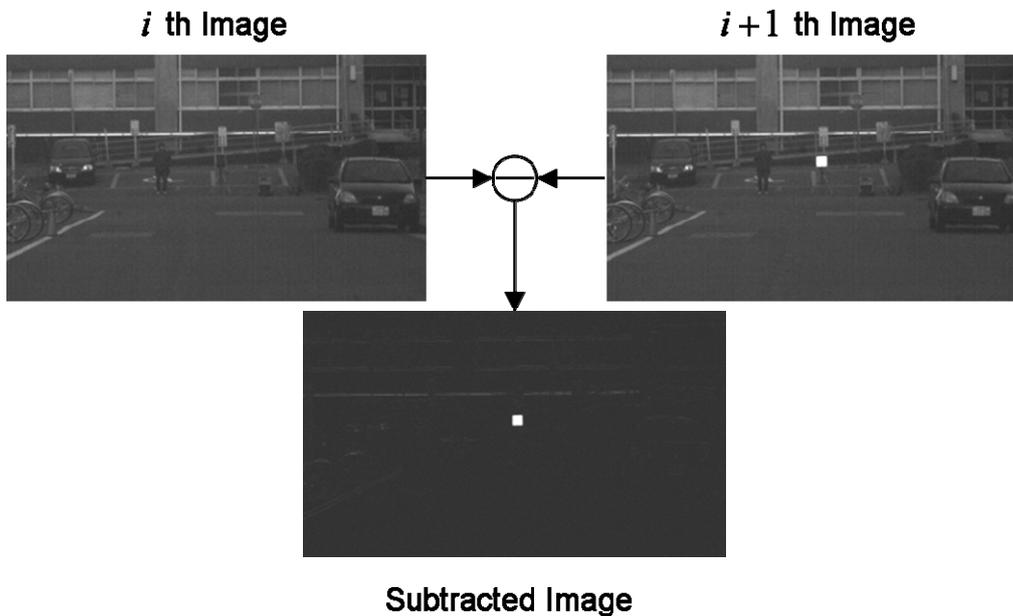
Figure 5. Resulted image by subtracting two successive images.
