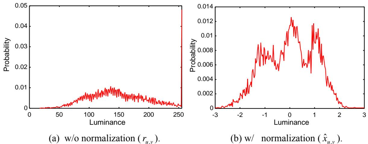
Figure 11. Received luminance distribution of the hierarchical coding (30m).
