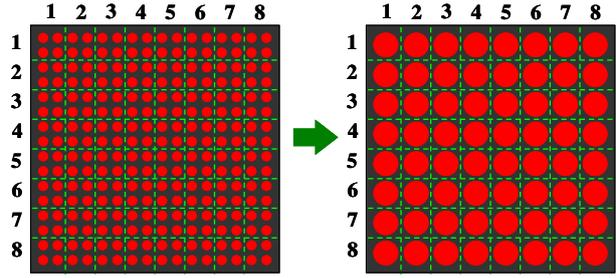
Figure 8. Representation of one data bit by 4 LEDs (2x2 LEDs)
