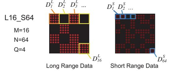
Fig. 8. Image of division of LED array.
