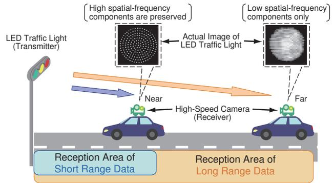
Fig. 1. Image of visible light communication using hierarchical coding.
