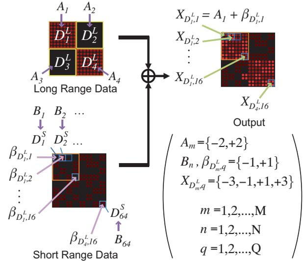
Fig. 4. Illustrated figure of the coding process.
