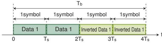
Fig. 5. Actual transmission data frame of one data.
