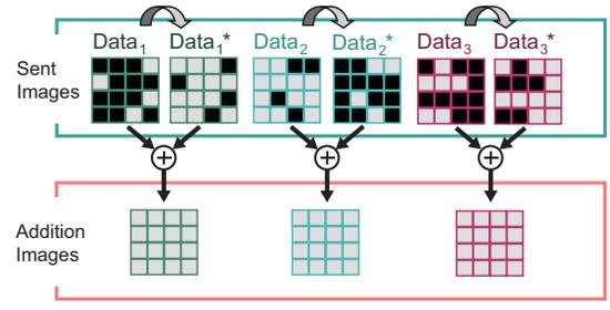
Fig. 6. Illustrated figure of the LED array tracking method using the inverted signals.
