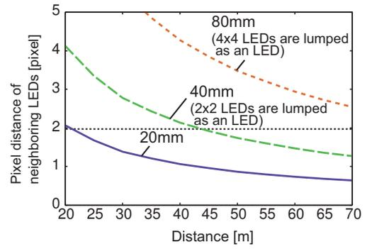
Fig. 3. Pixel-distance of neighboring LEDs versus transmitter-receiver distance, where the LED spacing is 20 [mm].
