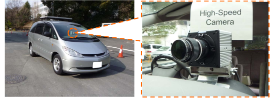
Fig. 8. Experimental equipment (receiver): On-board High-speed camera.
